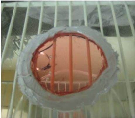
Ring of caulk on a 13" glass plate filled with fluid
